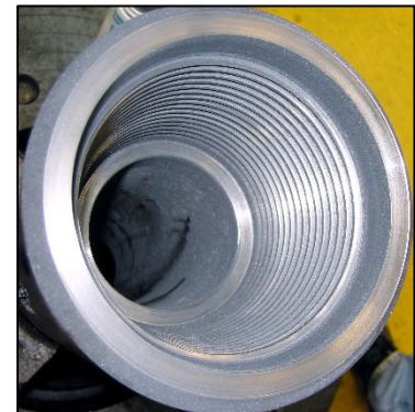
Example of clean threads & refaced shoulders
