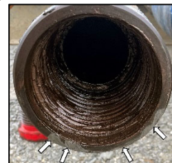
Seal face damage from Top Drive sub
