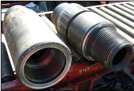
Example of seal face and thread damage
