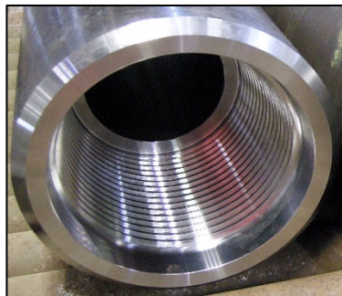
Example of good re-threading
