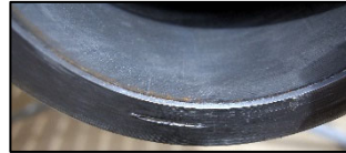
Example of seal face cut & protrusion
